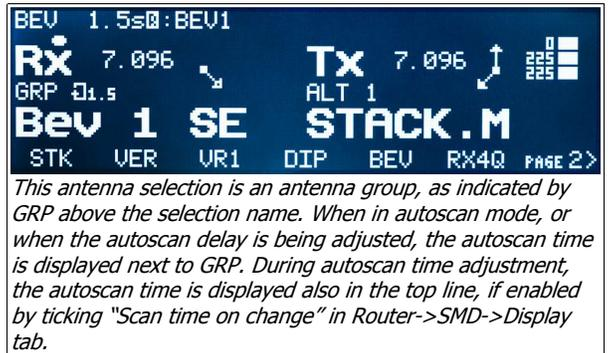
Automatic antenna scan and its features can be enabled/disabled via the FUNCtion menu.
