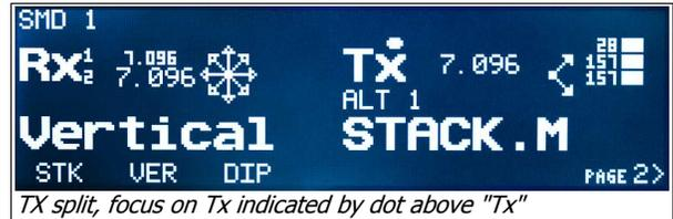
When PTT goes active (transmission starts), the focus is changed automatically to TX but it can still be changed by pressing the RX1-RX2-TX button. When PTT goes inactive (transmission stops), focus is returned to the state where it was before PTT went active.
