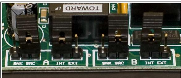
**NOTE:** The default factory settings for both PORT A and PORT B are INT / SRC (internal sourcing).
