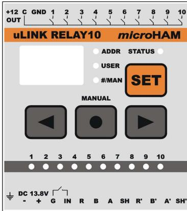
Every module has four (4) buttons, a set of status LEDs and a 3 digit display. Description below is valid for all modules.
