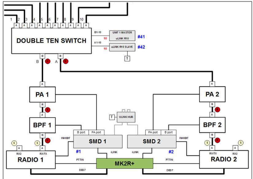
This configuration is the most common used by SO2R operators. However, it lacks the very useful ability to utilize the second receiver connected to separate antennas for diversity or “in band” split. The next example will examine how to get both two radio operation and dual receive.
