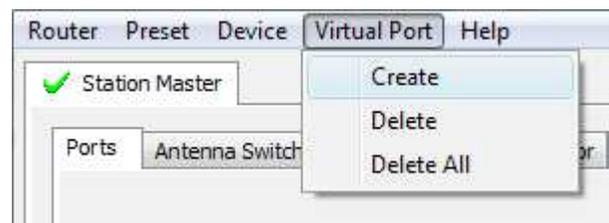
**Create** - Creates virtual COM ports. It is possible to select more than one port at a time by holding the *Ctrl* key on keyboard and clicking on COM port numbers. Creating virtual ports may take a long time (several tens of seconds), be patient.
