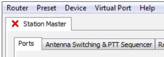
When Router shows a **RED** "X" instead of a green ✓, it means the device is disconnected and Router does not see the USB part of Station Master Deluxe. This happens when the USB cable is unplugged or the USB driver is not correctly installed.
