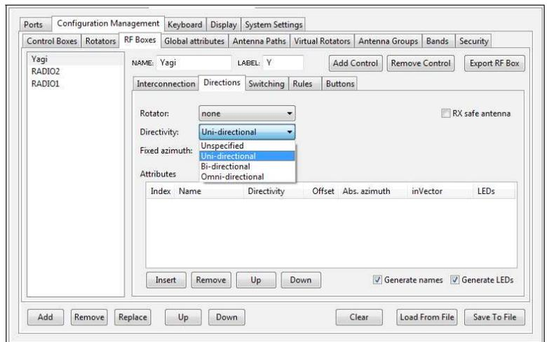
**WARNING:** Do not set this checkbox until you 100% sure there is sufficient isolation between any TX antenna and the **RX safe** antenna. In sufficient isolation may cause receiver damage!
