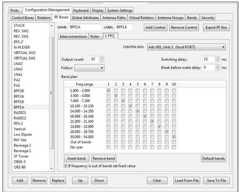
**FRQ** control allows a control box to be configured/used to control an RF box based on operating or transmit frequency. This is generally used for band selection.
