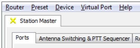
When Router shows a **YELLOW** "X" instead of a green ✓, it means the USB driver is correctly installed but Router can not communicate with the controller in Station Master Deluxe. This is usually because SMD is not turned on.
