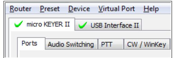
**Rename** – Creates a custom device name. This is useful if two or more devices are connected to the Router. For example CW KEYER, microKeyer and USB Interface II can be renamed to more identifiable names as shown here...
