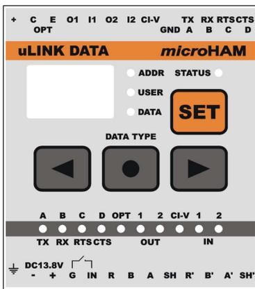
uLINK DATA is designed to control data devices and supports: one RS232 serial port with RTS/CTS, a CI-V port (translates frequency from the connected transceiver (SMD) to Icom protocol), two configurable inputs, two configurable open collector outputs and one optically isolated output.
