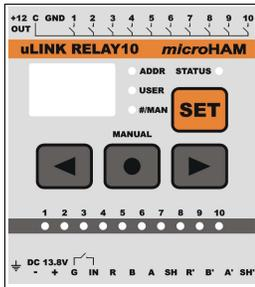
uLINK RELAY10 has ten (10) separate relay contacts and one common pole located at top terminal. Each contact is rated 3A/125VAC/30VDC. Common pole can be connected by external wire jumper to GND terminal pin for sinking outputs (connected to ground) or to +12 OUT terminal pin for 12V sourcing output. If controlled device requires different control power it can be applied to the C and GND terminal.
