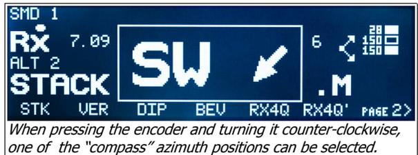
Alternatively, the target azimuth for rotators can be sent to SMD from any software capable of controlling DCU-1 rotators via the Router.
