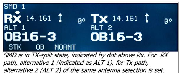
When switching to an antenna selection with alternate paths and a specific path is not available due to a conflict, the next free path is selected automatically. While using that antenna selection, the user can select among the other alternatives by repeatedly pressing the same selection button (1-7). The selected path is stored in the non-volatile memory. SMD will attempt to use the last selected alternative when returning to that antenna.
