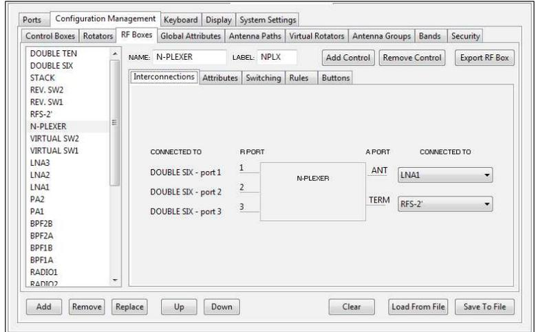
The TERM port cannot be left unconnected but also has no physical connection so it must be terminated by a “virtual” termination - in this case a “special box” called an “N-plexer terminator.” For convenience, it is wise to name each N-Plexer terminator the same as the antenna connected to the main port with an added apostrophe or other symbol to make it easy to recognize the master and mirror antennas.
