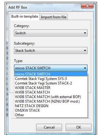
Because Stack Switch has three A ports, the first three bits represent A ports and another two BOP and FULL.
