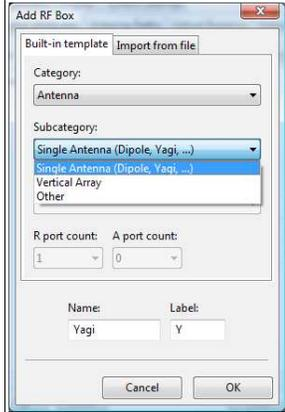
This type of RF Box allows adding R-port(s) only RF boxes – antennas to the configuration.
