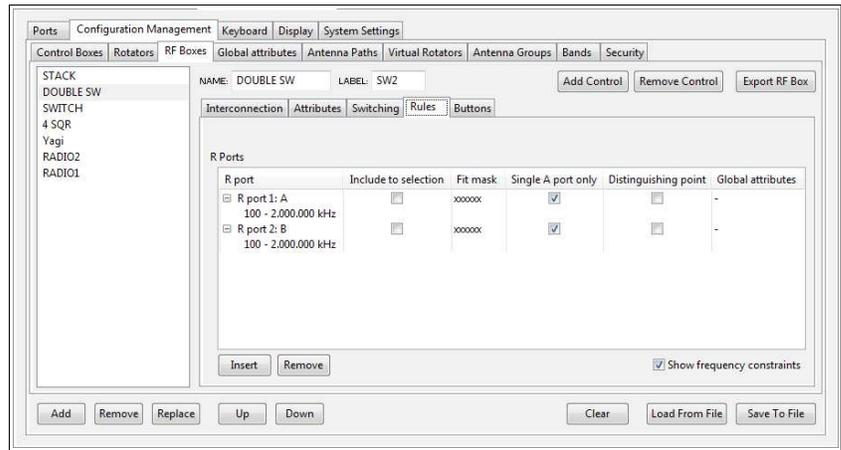
**IMPORTANT:** The control box for a double switch must control both R ports from within one relay unit.
