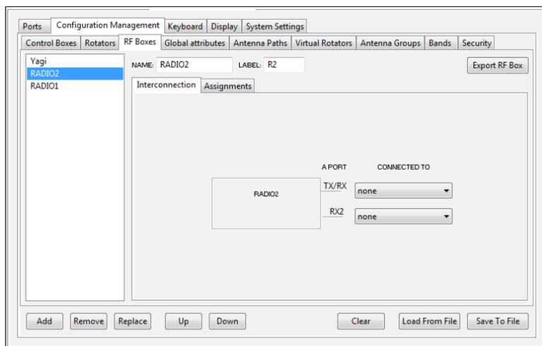
**Interconnections** tab specifies the (next) RF box to which the ports of the Radio RF box are connected.
