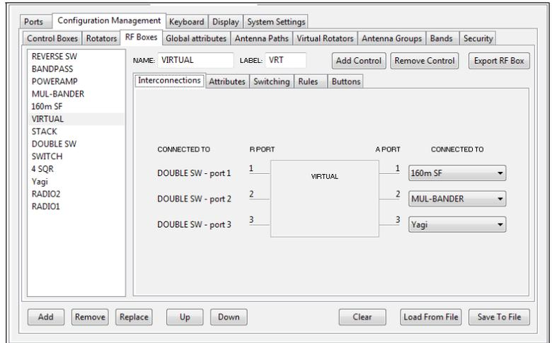
In our example we will insert a 3 x 3 virtual switch between the “real” antenna switch and the antennas. On the **Interconnections** tab we will connect the three A ports of the preceding “double switch” to the R ports of the virtual switch and connect the antennas to the A ports of the virtual switch.
