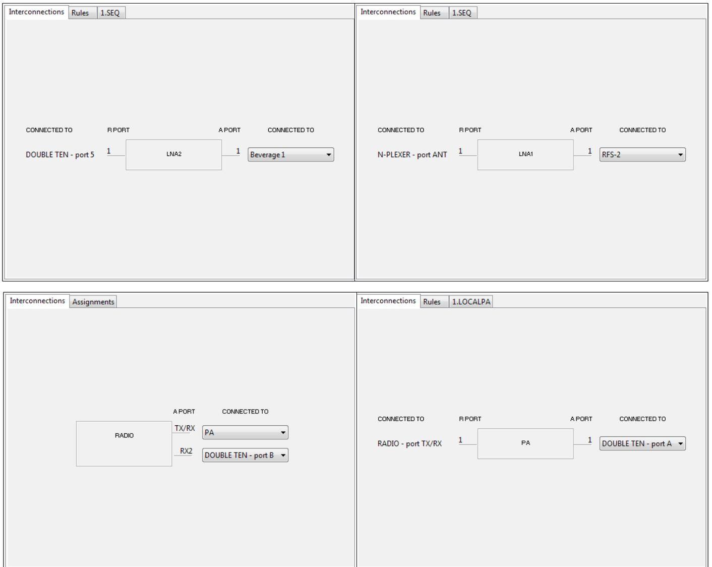
At this point about 95% of configuration work is already done. Clicking on any tab will cause Router to compile the configuration.
