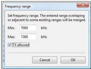
Frequency ranges can be quite complex, including separate frequency ranges for TX and RX Only. When a frequency range is specified with **TX allowed** box checked, the range is considered as valid for both RX and TX antenna path. If TX allowed is not checked, range is automatically considered as RX only and antenna path will not be offered among others TX antenna paths in this range. The picture above shows the frequency definition for 40/20/15/10m multiband antenna
