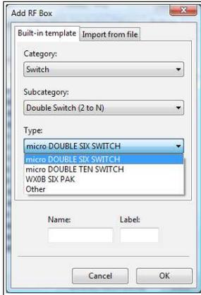
Double switches are special safety switches, originally designed for connecting two radios to several antennas. In our language, these are switches with two (2) R ports and several A ports. By design, the two R ports can not simultaneously select the same A port.
