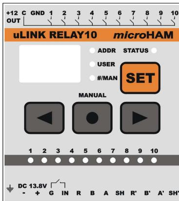
uLINK RELAY10 has ten (10) separate relay contacts **1 - 10** and one common pole **C** located at top terminal. Each contact is rated 3A @ 125VAC or 30VDC. The Left terminal, **+12 OUT**, is connected to the positive input (**+13.8V**) on the bottom terminal and **GND** is connected to the **Earth** pin of the bottom terminal.
