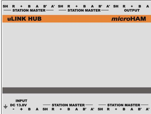
The uLINK HUB serves as a concentrator and isolated power source for SMD boxes connected to the uLINK bus. Up to four SMDs can be connected to one uLINK HUB. uLINK HUB is a basic element of the uLINK network and every setup must contain at least one.
