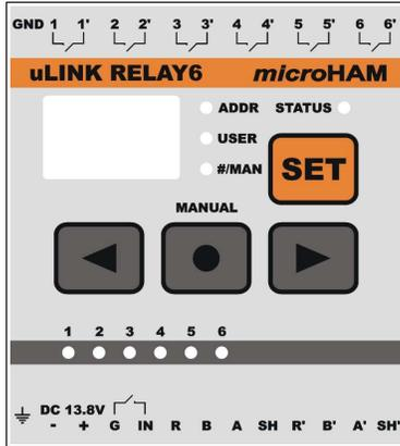
uLINK RELAY6 has six (6) isolated SPST contacts **1 – 6** located at top terminal. Each contact is rated 3A @ 125VAC or 30VDC. The left (**GND**) terminal is connected to the Earth pin of bottom terminal.
