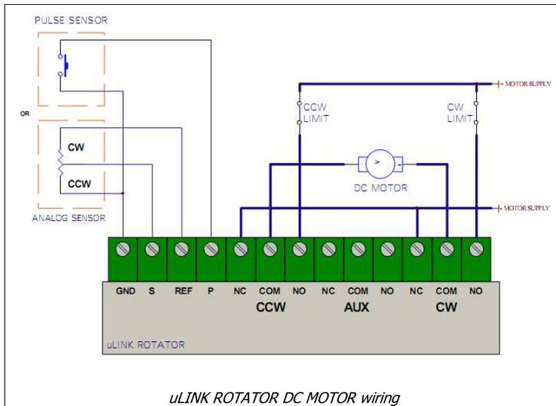
Each SPDT relay contacts for CW, CCW and AUX are located on top terminal.
