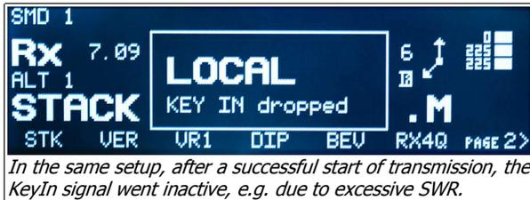
In addition, some specific, permanent reasons for TX disable may result in more descriptive messages - "INHIBIT raised", "KeyIn timeout", etc. - and the number of the offending unit where appropriate.
