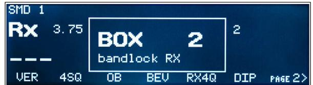
If "Detach RX antenna" protection is selected, the message "BOX [nr of other SMD] - bandlock RX (or RX2)" is displayed on the SMD receiving on a band where other SMD started to transmit, while its RX path is disconnected. If the offending SMD subsequently leaves this band, a "BOX [nr of other SMD] - left RX (or RX2) band" message is displayed.
