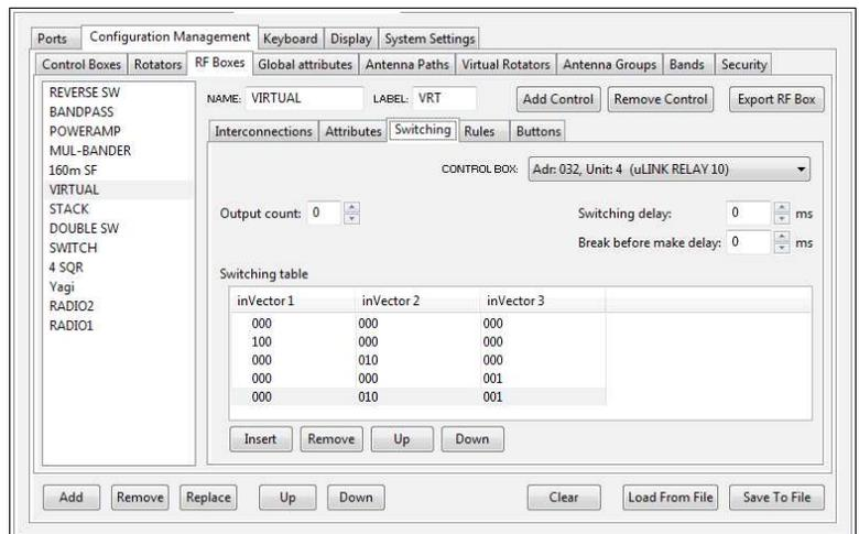
In our case, InVector 100 000 000 means that when R port 1 (160m) is used, the other A ports must be off (first 100 part) and the other R ports may not be used (000 of other two parts). When R port 1 is not engaged, R ports 2 and 3 can be freely used. This gives three possible combinations: tribander only (000 010 000), 80m Yagi only (000 000 001) or both by separate radios (000 010 001). All combinations **must** be explicitly defined. Masks are not allowed for virtual switches.
