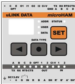
uLINK DATA is designed to control data devices and supports: one RS232 serial port with RTS/CTS, a CI-V port (translates frequency of the transceiver coupled to SMD into the Icom protocol), two configurable inputs, two configurable open collector outputs and one optically isolated output.
