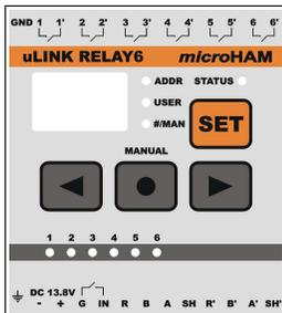
uLINK RELAY 6 and uLINK RELAY 10 are the most used uLINK network module – they provide relay contact outputs for device control. The relay modules are used for any device requiring simple control – switch input to ground, connect to power or connect two input ports together. uLINK RELAY6 has six (6) isolated SPST contacts located at top terminal. Each contact is rated 3A @ 125VAC or 30VDC.
