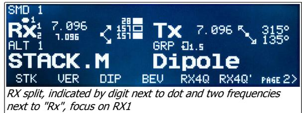
The list of available selections changes according to the current focus (LCD display, pos.11).
