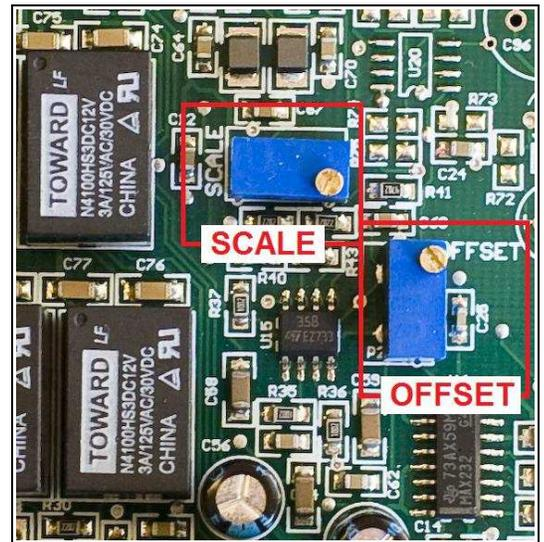
11. Slightly readjust SCALE trimmer for improved accuracy until sensor value shows 1021 (between 1020-1022) and click next.
