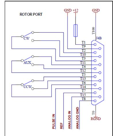
To the right are examples of the connection for home brew AC and DC motors. Only one type of position sensor is needed. For analog systems, 500 ohms provides proper power supply loading and optimum immunity to RFI. However, any value from 500 to 5K ohm is acceptable.
