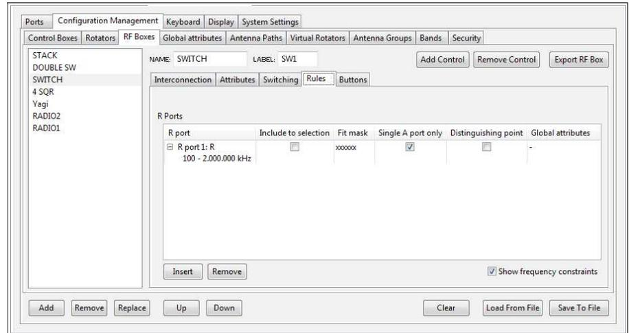
**Include to selection** checkbox has the same meaning as for antennas or two port devices. When checked, the R port will be added as a separate antenna selection for direct access from the SMD main antenna selection buttons. Since a simple N way switch will most likely have antennas or additional switches connected to its A port(s), the default value is that R port of an N way switch is not included in the available antenna selections.
