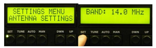
Then we select how many antennas we want per current band (1 or 2) always confirm your selection by pressing SET. The by scrolling UP / DWN you assign which PORT is used on your external antennas switch for this particular antennas. (ANT 1 ON PORT 01)
