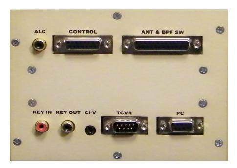
**KEY IN**- Input signal PTT (switching voltage / current 5V / 2mA) **KEY OUT**- Output signal PTT (maximum switching of 30V / 50mA)
