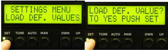
Then we select if want to erase all settings (pressing TUNE) or just one settings parameter (SET button). In case we are defaulting just single parameter use UP / DWN to select which option and confirm by SET.
