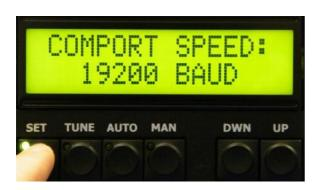
By scrolling UP / DWN select desired Baud Rate which must be same as baud rate used by connected TRX.( please refer to your TRX user guide)To confirm your selection press SET. When using Yaesu TRX you need to configure STOP BITs parameter and confirm selection with SET.
