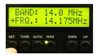
To enter Manual mode of the PA please press MAN. By pressing MAN repeatedly you select BAND and band's segment You can control the segment or band by scrolling the UP / DWN buttons.
