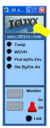
Make sure you have properly connected the RS232 cable and have installed the software that came with P. A. "RF Amplifier Monitor".
